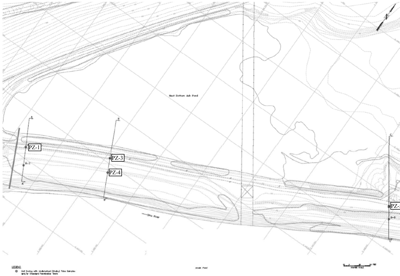
FIGURE 1. WEST BOILER SLAG POND PIEZOMETERS LOCATION PLAN
